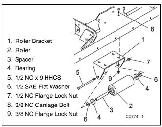
Figure 32. Front Roller Installation
